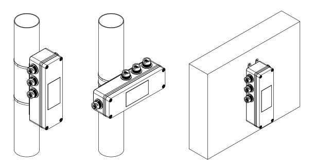
DCMD-4I is available for ordering with included pole mount kit, which allows easy install on any pole with diameter over 50mm vertically (recommended method) or horizontally. If necessary - DCMD-4I is also available with included wall installation kit.
